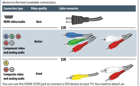
HDMI-to-DVI adapter to the end of the HDMI cable that connects to the DVI device's jack.
